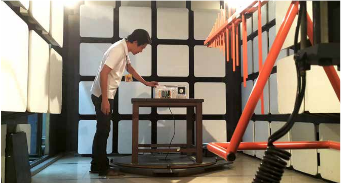
Delta Engineer performing Radiated Emissions Test Process
