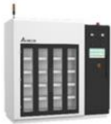
Energy-Recycling Burn-in Chambers
