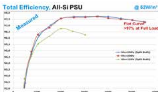
Efficiency curve over load of the All-Si PSUs (6000W & 3000W variants) employing cost effective standard Mosfets.
