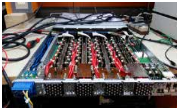
AC/DC Power Shelf for open19.org with 19,2kW 50 fused 12V outputs
