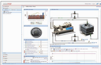
Building Management System (enteliWEB)
